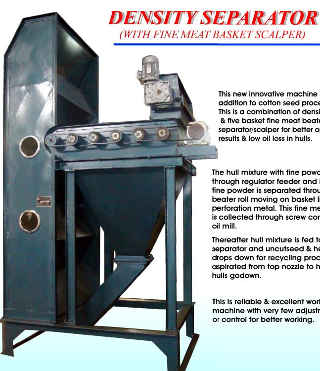
This new innovative machine is a latest addition to cotton seed processing plant. This is a combination of density separator & five basket fine meat beater separator/scalper for better operational results & low oil loss in hulls.
